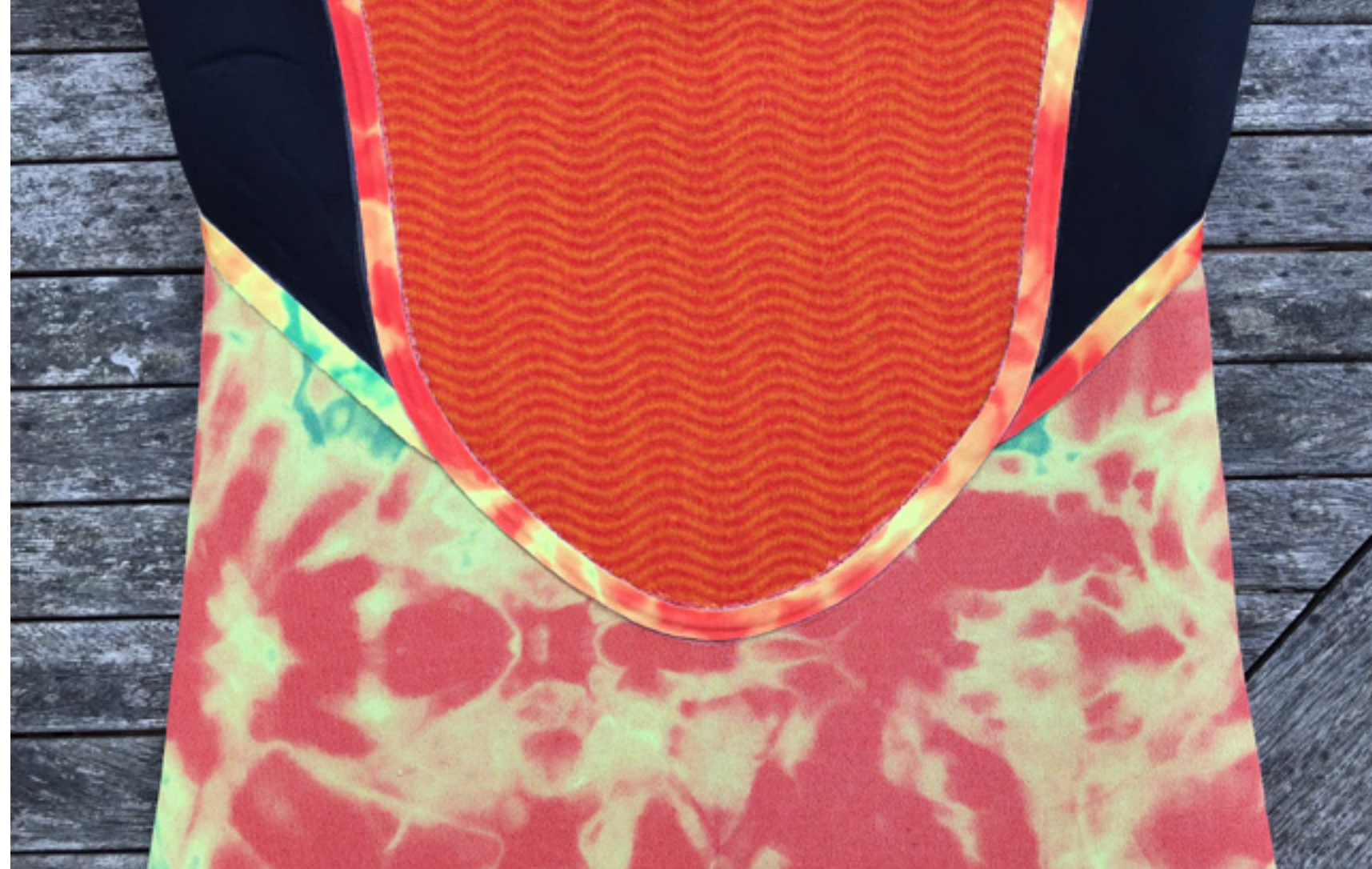
Three different types of insulative interior lining on the XCEL Revolt wetsuit
